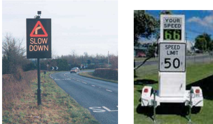
Figure 15: Examples of Vehicle Activated Signage
