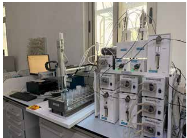
Fig. 57 Automated water chemistry system
