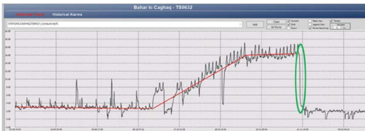
Figure 54 Snapshot from SCADA showing conductivity of the wastewater received by Bahar iç-Çağhaq PS for the period 01-09-25 to 04-12-25
