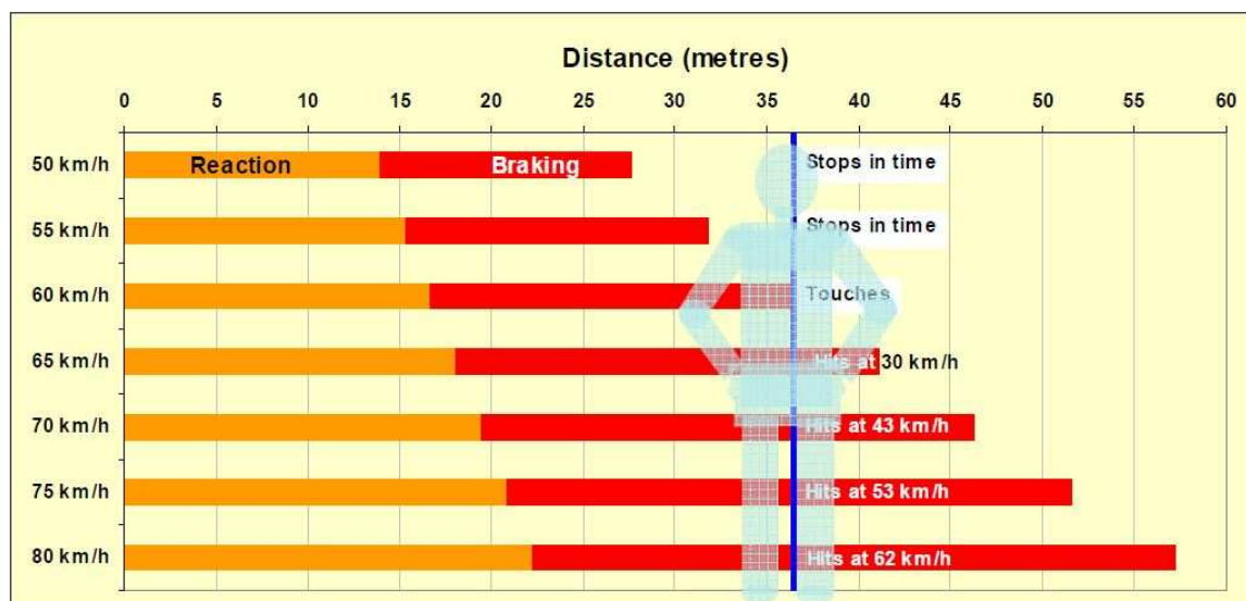
Figure 1: Vehicle stopping distances at different speeds
